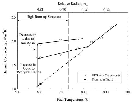
Figure 16: Thermal conductivity of the high burnup fuel at  $217^{\circ}C$  as a function of the local radial temperature during the last irradiation cycle. At  $r/r_0 = 0.81$ , where the local burnup was 90 MWd/kgHM, the local thermal conductivity of the fuel rod would have been 20% higher in the absence of gas pores. 5 % porosity is a hypothetical value equating to the porosity of the fresh fuel [50].
