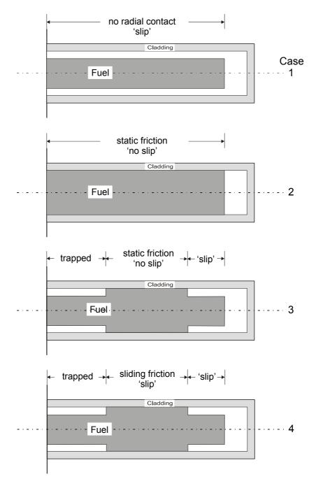
Figure 10: Four possible modes of an interaction between fuel and cladding.
