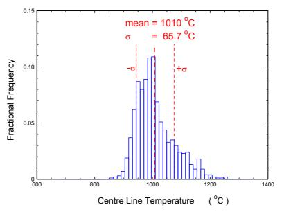
Figure 15: Fractional frequency of the centre line temperature predictions, when varying only three input parameters  $(q', h_{gap}, \lambda)$ .
