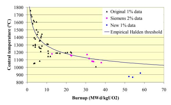
Figure 12: Original Vitanza criterion for the onset of fission gas release and supporting data [29,30].
