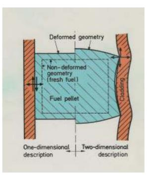
Figure 1: Schematic view of a deformed fuel pellet; comparison between a onedimensional and a two-dimensional description.
