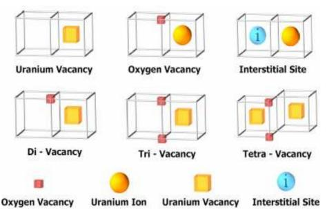
Figure 11: Possible solution sites for fission products in  $\text{UO}_{2 \pm x}$  according to Grimes [25]
