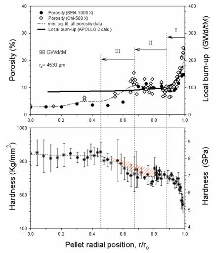
Figure 17: Experimental values for micro-hardness of irradiated  $UO_2$  fuel with a burnup of 98 GWd/tHM [51]
