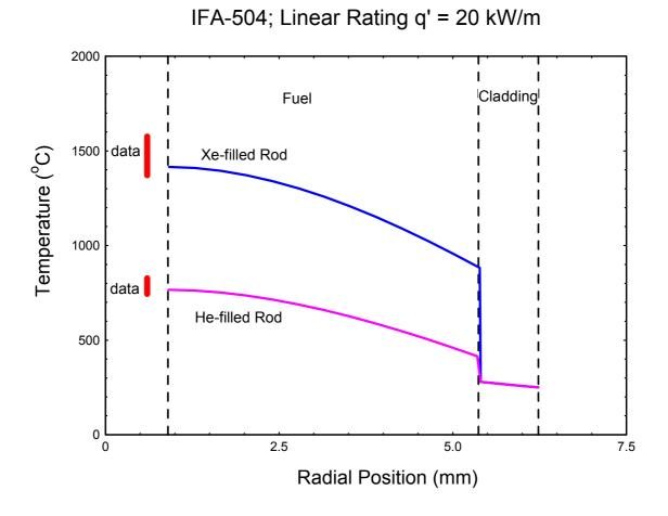
Figure 3: Radial temperature distribution in a BWR-rod at begin of life. Comparison between the range of experimental results and predictions of the TRANSURANUS code for two different fill gases (He, Xe). The data refer to a thermocouple measurement in the central hole of the fuel pellet, indicated by the dashed line.
