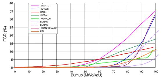
Figure 19: Cumulative fractional fission gas release predicted for a constant linear heat rate of 15 kW/m by various fuel performance codes involved in the FUMEX-II round robin exercise of the IAEA [60]
