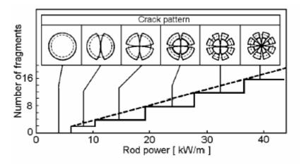
Figure 6: Calculated crack pattern from thermoelastic stress [19]
