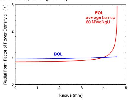
Figure 2: Radial form factor of the power density  $q^{m}$  at beginning and end of life for "typical" LWR conditions according to the TUBRNP model [8]. The radial distribution of the power density depends on enrichment, rod diameter, neutron spectrum and other parameters.
