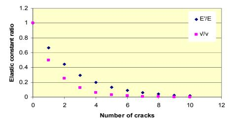
Figure 9: Effect of the number of cracks on the elastic modulus and the Poission's ratio according to Jankus et al.[23]
