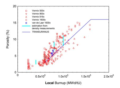
Figure 20: Porosity as a function of the local burnup for highly irradiated fuel, and the corresponding correlation adopted in the TRANSURANUS code [61].
