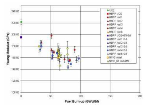
Figure 18: Experimental Young's modulus of irradiated LWR fuels as a function of burnup [56].
