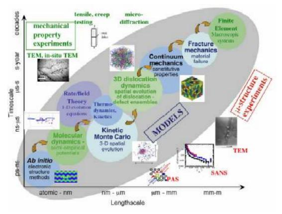
Figure 24: Illustration of an integrated experimental and computational approach to the multi-time-scale investigation of materials behaviour [74]. A number of microstructural characterisation techniques important for validating model predictions are also represented: Positron Annihilation Spectroscopy (PAS), Small Angle Neutron Scattering (SANS), Transmission Electron Microscopy (TEM).
